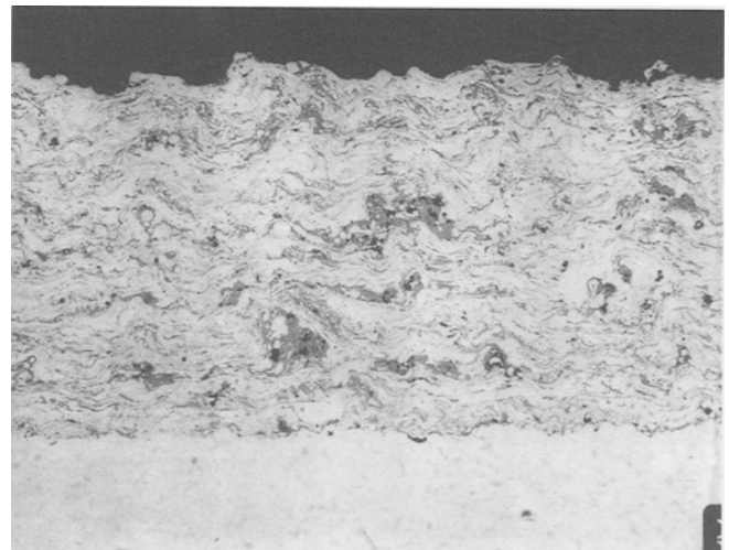
Fig. 2 Cross section of carbon steel molten droplets sprayed with pure nitrogen and quenched in a bath of liquid nitrogen
